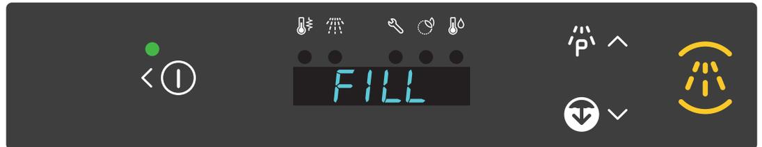
Once the filling process is completed, the heating process begins and the chemical dispensing process (if applicable)
