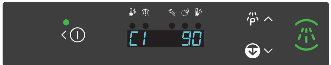
If however, a minimum wash temperature has been set (this function can be enabled only by an authorised technician) and the temperature in the tank is inferior to the set temperature, the dishwasher will move on to the heating phase and the display will read HEAT with intermissions of the temperature displayed:
